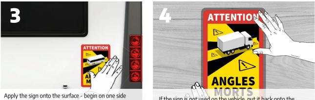
and smooth the film sheet down to the other side. Repeat the wiping movement with increased pressure
