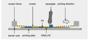
Before starting the screen printing process, the screen, squeegee and flood bar must be cleaned with a suitable solvent. In addition, each film should be wiped with an anti-dust or anti-static cloth prior to printing.
