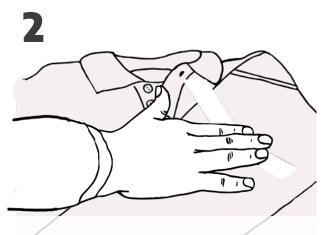
Place the reflective film on the substrate with the adhesive side down and cover the reflective side with a press cloth.
