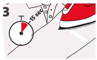
Set the iron to 165° C and press it for about 15 seconds evenly onto the fabric (no steam).
