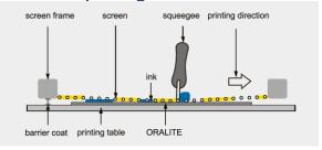
Before starting the screen printing process, the screen, squeegee and flood bar must be cleaned with a suitable solvent. In addition, each film should be wiped with an anti-dust or anti-static cloth prior to printing.
