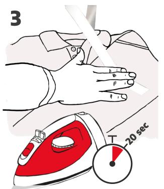
Place the reflective transfer film on substrate with the adhesive side down and evenly press the iron onto the substrate for approx. 20-25 seconds (150-160 °C) without using steam. Please use a non-stick slip sheet between iron and laminating surface.
