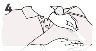
Allow application to cool to room temperature before removing the liner covering the reflective side.
