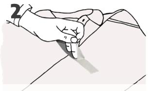
Remove transparent adhesive side liner exposing dry adhesive. Do not remove reflective side liner.
